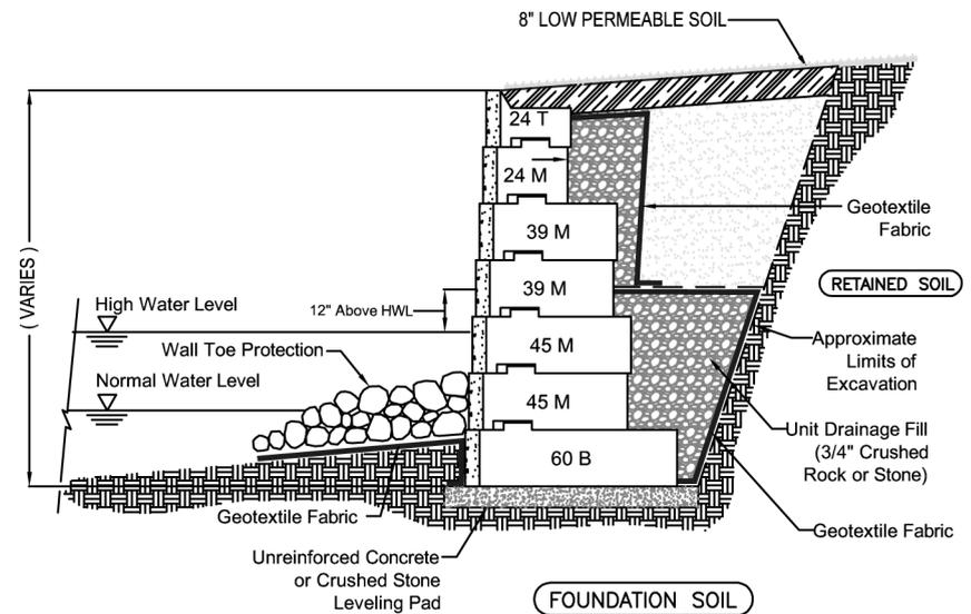
Typical Gravity Water Wall Section
