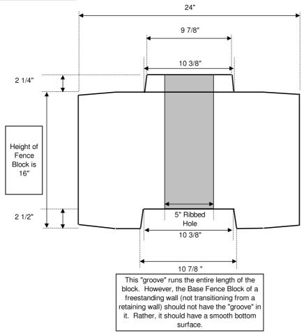
The knob on the top of the fence block actually represents 2 circle knobs 10 3/8" in diameter at the base of the circle and positioned so that the center point of each knob is 24" apart from each other. See Top Down View for spacing details. Also, a smaller ribbed hole (5" in diameter) will be cast in the center of the knob to allow for vertical reinforcement of the wall.
