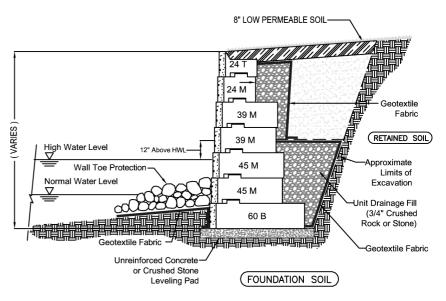
Typical Gravity Water Wall Section
