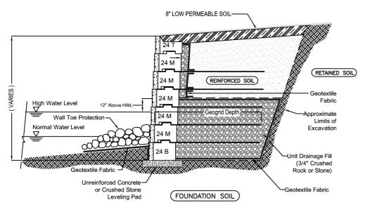
Typical Reinforced Water Wall Section
