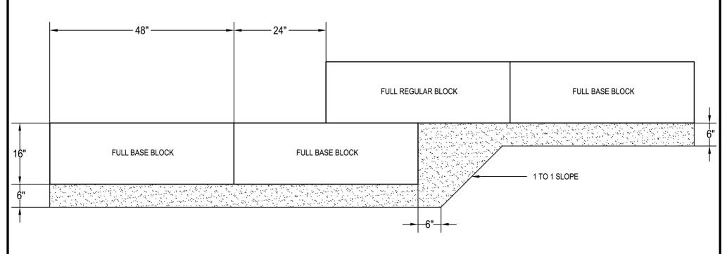
NOTE: BLOCK MUST BE PLACED ON A MINIMUM OF 6" OF CRUSHED STONE (GENERALLY 3/4" DOWN OR CLASS 5) OR LEAN CONCRETE AS SPECIFIED IN THE SITE SPECIFIC WALL PLAN DESIGNED BY A REGISTERED PROFESSIONAL ENGINEER. GENERALLY THE BASE MATERIAL MUST BE COMPACTED TO 95 PERCENT OF STANDARD PROCTOR.
